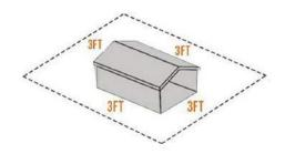
A minimum of 3 FT level clearance around the entire building (clear of any vegetation or debris) is required for install.
